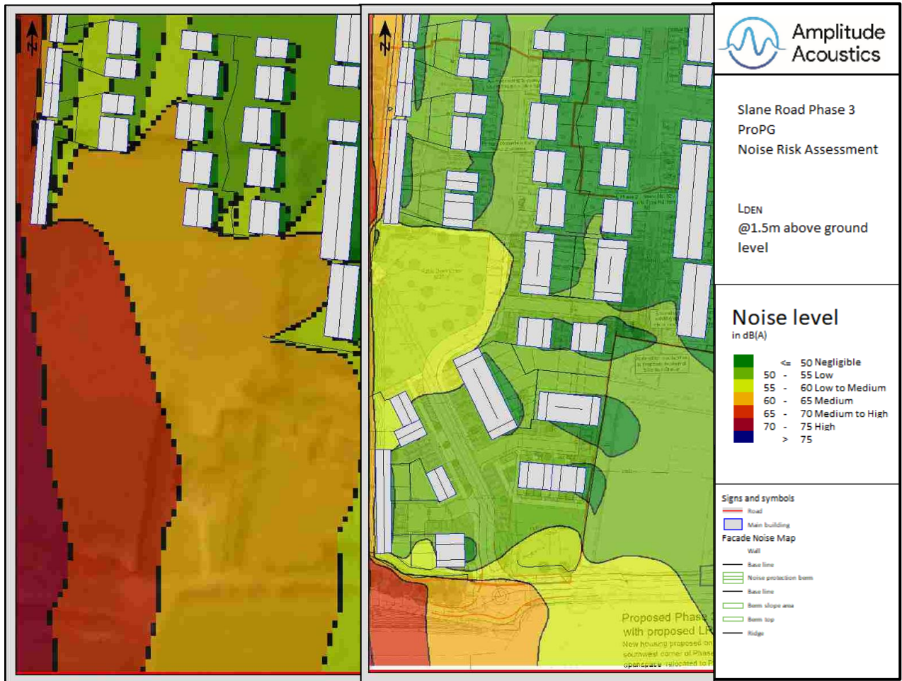
Figure 3. Side-by-side comparison of predicted L DEN road traffic noise contour bands for the existing site without (left side) and with (right side) the development in place. (Scenario 2035)
